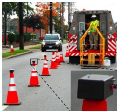
Figure 1: Our sensornet system deployed in a work zone to measure traffic. The nodes are mounted on top of construction safety cones. The placement of the cones is as required by the work zone itself as per the MUTCD [1].
