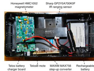
Figure 3: The sensor node that we deploy in the work zones. The node include a TelosB mote, with a Telos charger board connected to rechargeable batteries. The mote is connected to the Sharp IR ranging sensor, and an EasySen sensor board which includes the Honeywell HMC1052 magnetometer.
